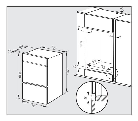
To ensure adequate ventilation to the oven once installed:
